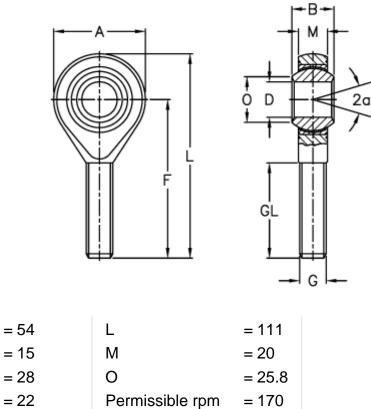
Static load C0 (kN) = 100
